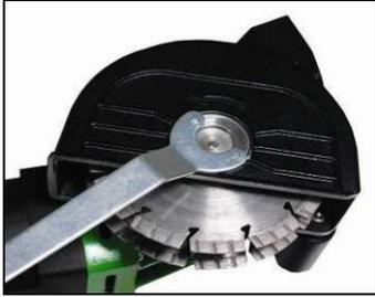
Open the clamping screw with the face spanner and remove the diamond cutting discs as well as the spacer discs from the work spindle.
